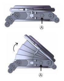
It is necessary to press and hold the deployment lock (A) of the Opera located at 9 o'clock on the bezel and then open the case by grasping it from above and gently pulling it.
