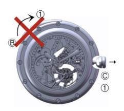
Be careful never to lift the lock of the minute repeater (B) in position (1) when the winding stem (C) is pulled into position (1).
