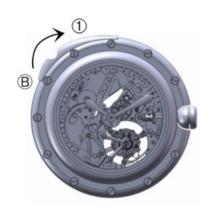
The trigger (B) of the Opera located at 9 o'clock on the bezel allows the minute repeater mechanism to be armed. To do so, it must be pulled to the full towards 11 o'clock and then released. Once the hours, quarters and minutes have been rung, allow the mechanism to fully discharge for at least 30 seconds.
